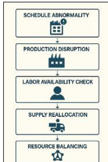
Figure 3 “Example of Real-Time Resource Balancing Workflow in a Production Environment,” illustrates how live data feeds enable system-level synchronization of equipment load, labor deployment, and material delivery pacing. Integration between ERP procurement triggers and MES floor execution allows procurement adjustments to occur in near-real time when material constraints are detected, thus preventing shortages before they impact workflow [30]
