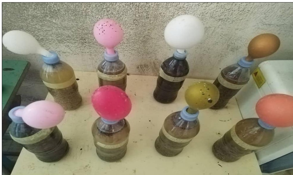
Figure 4 Biogas productions after one week
