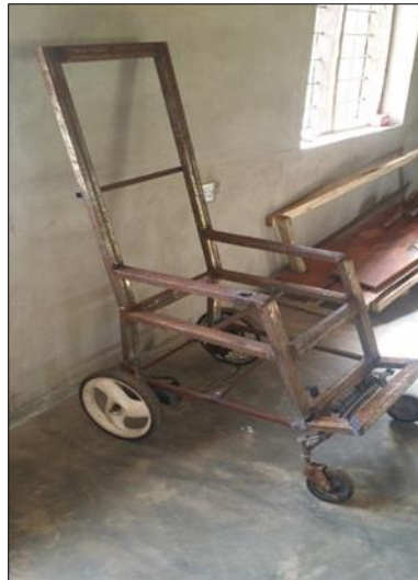
Figure 4 Smart wheelchair frame construction
