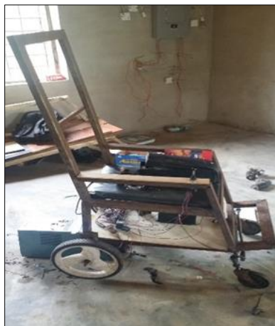
Figure 5 Smart wheelchair electrical construction
