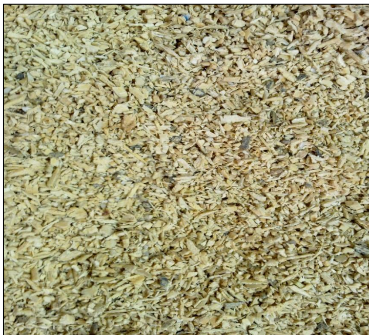
Figure 1 Shells of Balanites aegyptiaca (L.) Del. after crushing and sieving
