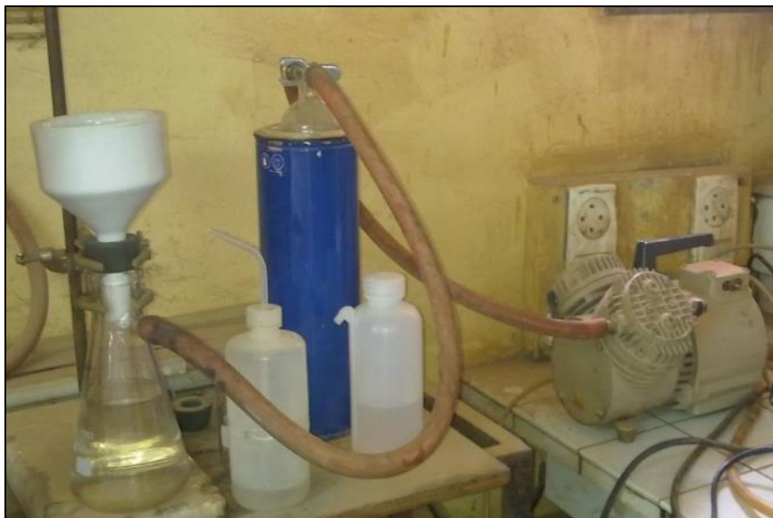
Figure 3 Filtering the sample on a Büchner funnel
