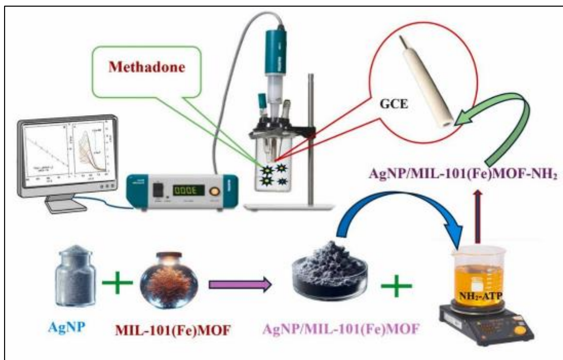
Figure 12 Schematic illustration of the hydrothermal synthesis of MIL-101(Fe), its post-synthetic functionalization with silver nanoparticles (AgNPs) for enhanced conductivity, and ATP for biomolecule affinity
