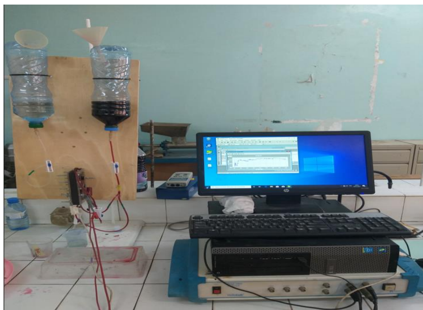
Figure 2 Experimental setup for the continuous electroreduction of Hibiscus sabdariffa L extract
