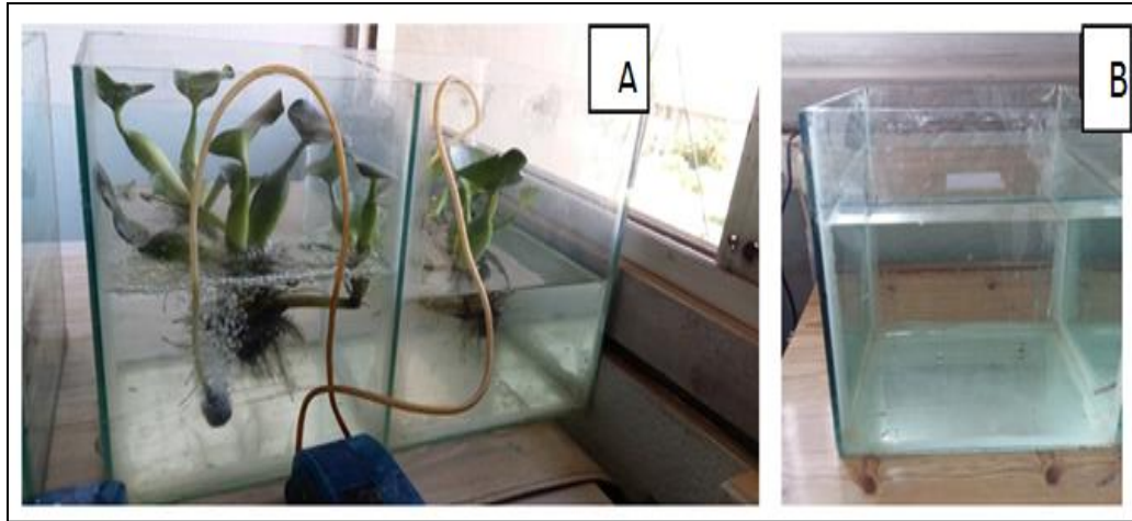
Figure 4 Control ponds (A) contain a water hyacinth plant without treatment to estimate the rate of transpiration (B) a pond without a plant contains only water to estimate the amount of evaporation
